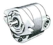
The CROSS Series 50 gear pumps feature a gear tooth design that provides more displacement within a given package size. Available in 7 sizes, with displacements from 1.52 to 5.20 cubic inches per revolution, this compact pump can deliver up to 45 gallons per minute in a space less than  $6^{1}/_{2}^{11} \times 5^{3}/_{4}^{11} \times 7^{1}/_{4}^{11}$ . Gear tooth design and pressure-balanced loading plates provide high volumetric and overall efficiency while operating at a low noise level.
